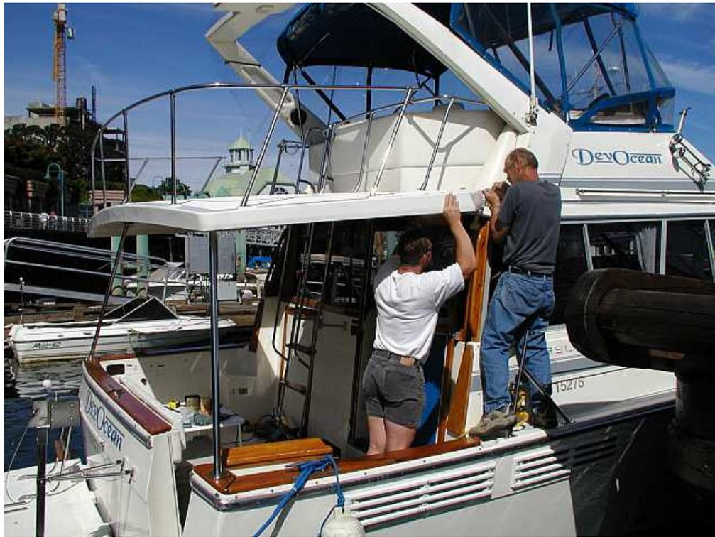
5. Align companion way opening in hardtop with existing ladder opening in cabin top. Make sure hardtop is not twisted to port or starboard. Sight down hardtop sides and make sure hardtop is square to cockpit sides. The opening in the hardtop for the ladder should be as far forward as possible. Approximately 5 to 5 1/2 inches of the hardtop flat flange should rest on the existing cabin roof. Clamp in place. Re check alignment.
