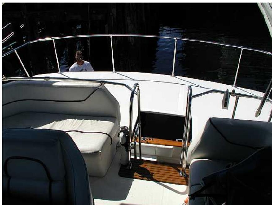
6. Drill  $\frac{1}{4}$  inch holes through hardtop forward flange and cabin top on either side of the ladder opening. Drop in  $\frac{1}{4}$  inch bolts to maintain alignment. Drill 3 more equally spaced  $\frac{1}{4}$  inch holes to port of the ladder opening and 5 more equally spaced holes to starboard of the ladder.
