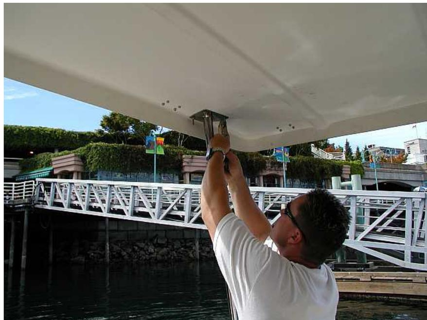
**Note:** The stanchion mounting plates may need to be pounded with a heavy hammer to make them align with the wood transom cap or the underside of the hardtop. **Use a block of wood between the hammer and the stanchion mounting plate.** Do this while the bolts are being tightened
